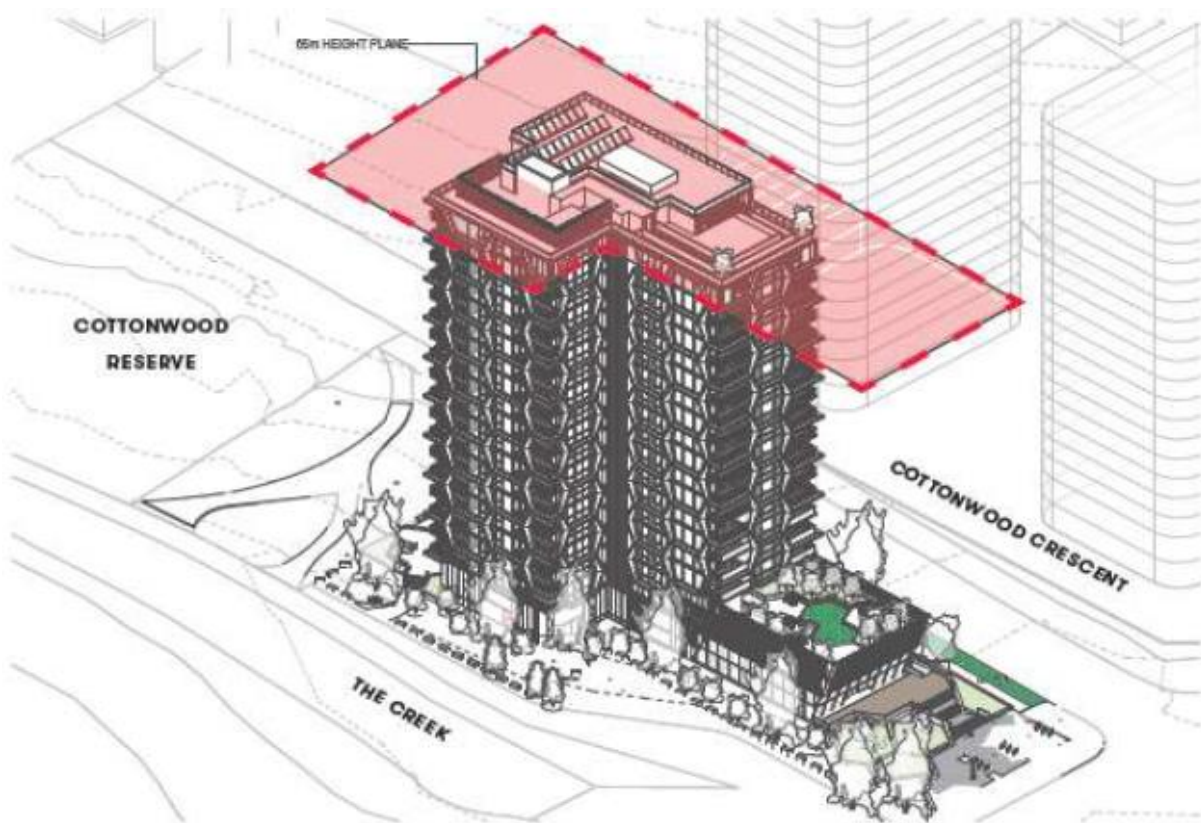
Figure 20: Massing diagram with building height plane showing non-compliant plant and lift overrun (Source: Scott Carver, Drawing AD-DA3991).
